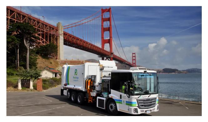
Recology has used the Hyzon and New Way's hydrogen fuel cell refuse collection vehicle on normal routes in San Francisco, putting it through a full day with about 600 residential waste bin lifts. The truck has so far tackled a 27% grade on the hilly city's streets. The truck lasted multiple service days on a single fueling of its hydrogen tank. In contrast with battery-electric trucks Recology has used, the hydrogen fuel cell truck doesn't have an issue with heavy payloads.
